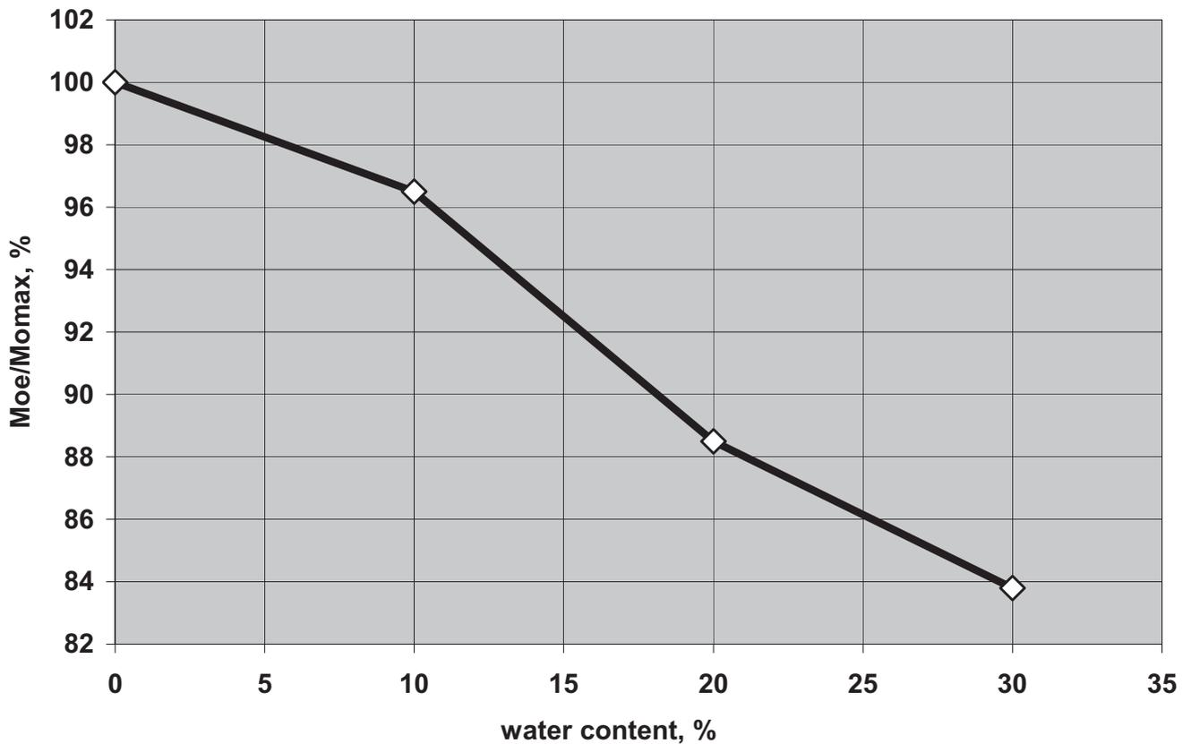
Fig. 4. The effect of water proportion in the emulsion fuel on the relative value of the engine torque
