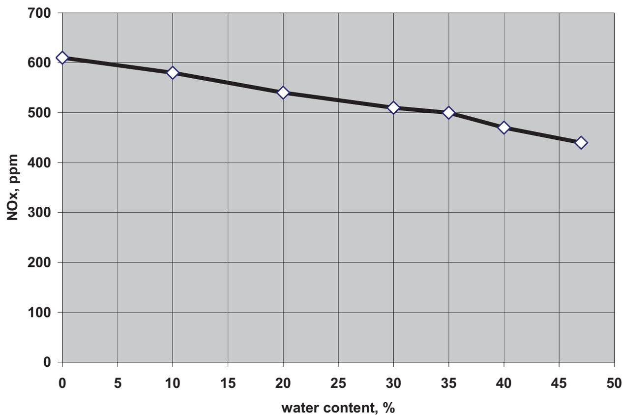
Fig. 2. Concentration of NOx in exhaust gases in the function of water proportion of water injected to the suction manifold [6]
