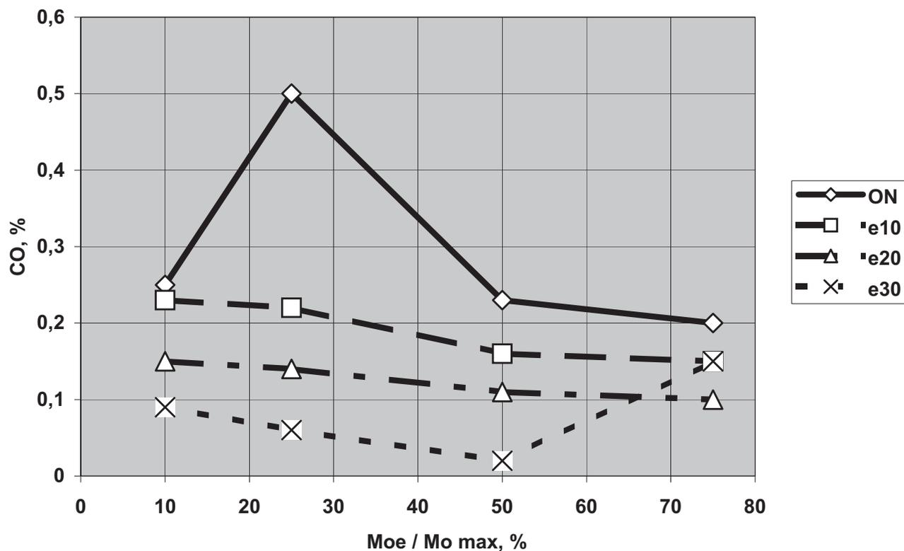
Fig. 5. Concentration of CO in exhaust gases in the function of the engine load for different water proportions in the emulsion fuel: ON – diesel oil, e10 – 30 emulsion fuel of water content 10-30%
