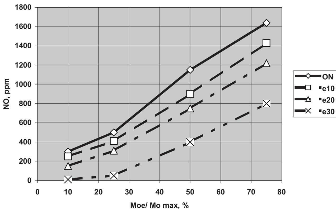
Fig. 6. Concentration of NO<sub>x</sub> in exhaust gases in the function of the engine load for different water proportions in the emulsion fuel: ON – diesel oil, e10 – 30 emulsion fuel of water content 10 – 30%
