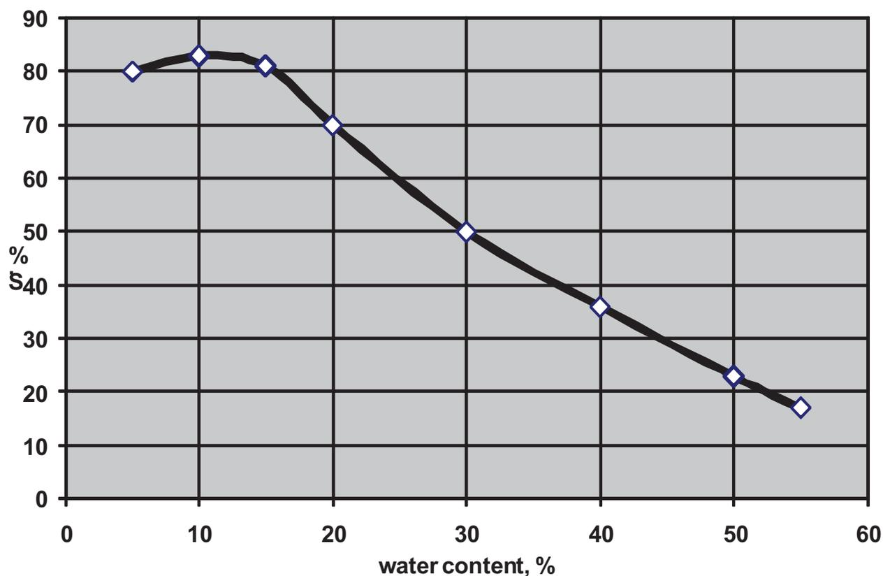
Fig. 1. The effect of water proportion in fuel on the change of the engine smoking [1]
